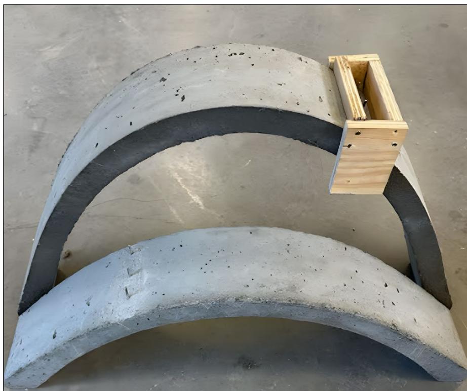
Figure 12 Steep and shallow arch geometries with the formwork required for the bearing surface for the eccentric load application
