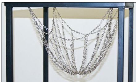
Figure 5 Bradley and Gohnert (2016) used this hanging chain model to describe the inverted catenary form of a vaulted structure
